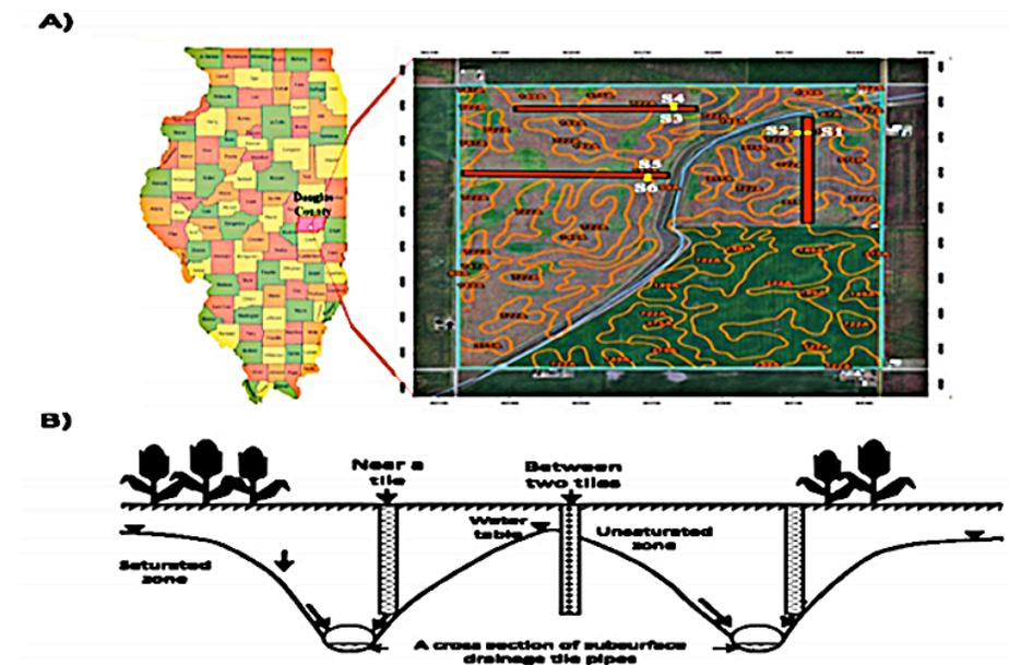
Fig. 1: A) The sampling location at a Douglas county study site (39°43'01" N, 88°14'01" W) in east-central Illinois. Filled red rectangles and filled circles represent tile lines and sampling locations for soil 1-6 (S1-S6), respectively; B) sample location description of selected tile lines: S1, S3, and S5 are near a tile; S2, S4, and S6 are between two tile lines. They are about 15m apart of each other.
