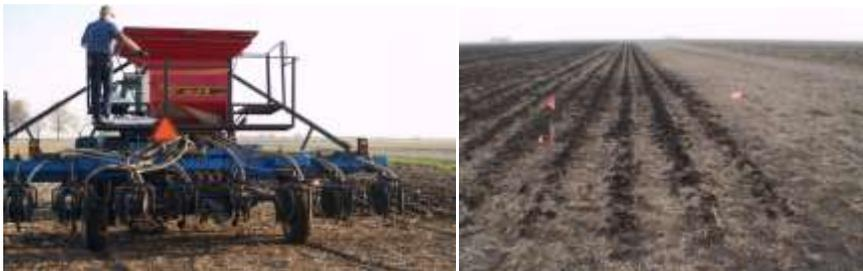
Photo caption: [left](#)) DMI Model 4300 Strip-till tool bar with Gandy Orbit-Air dry fertilizer box, [right](#)) Strip-till ridges following fall application.
