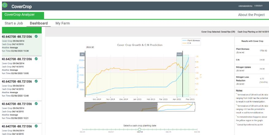
The visualized output in the dashboard is the product of running DSSAT in the web environment using information for actual fields; data input by the user, such as management, as well as weather and soil data. The user begins by selecting an actual field from a mapping tool, as demonstrated in Figure 2.
