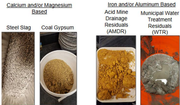
Figure 4. Phosphorus sorbing materials being characterized. Image from Berkshire, T., R. Christianson, L. Christianson, A. Margenot. 2018. Removing Dissolved Phosphorus with Edge-of-Field Phosphorus Filters. Illinois Nutrient Loss Reduction Strategy Partnership Workshop. Champaign, IL. Newer results will be shared in San Antonio in November 2019.
