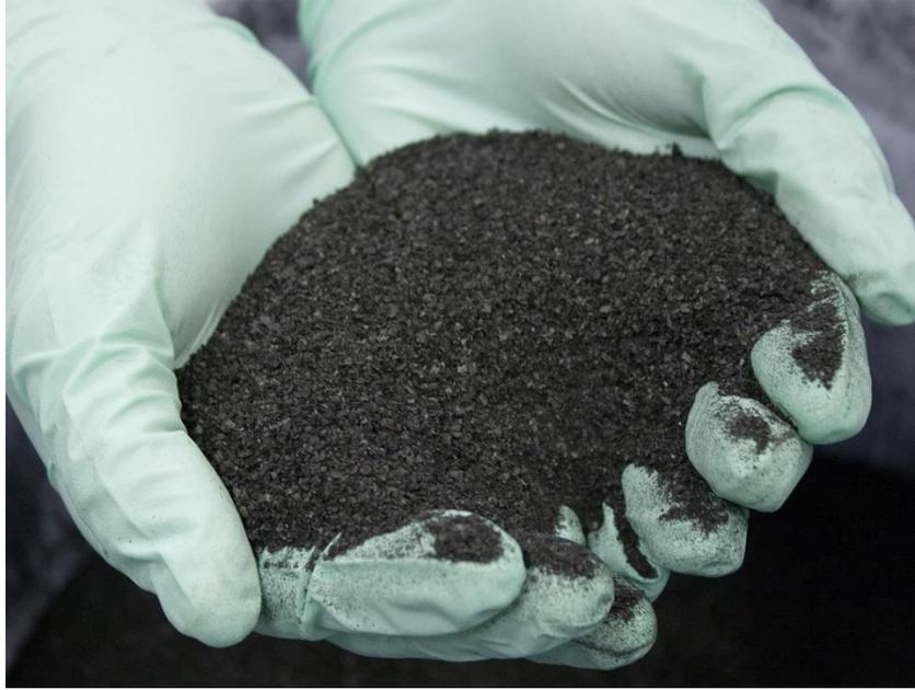
**Figure 1.** Biochar produced from sawdust via pyrolysis
