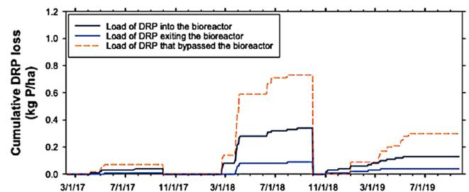
*Dudley Smith Farm bioreactor cumulative dissolved reactive Phosphorus (DRP) loss entering, exiting, and by-passing the bioreactor. Loads restart at the water year (October 01) and the three annual periods have DRP loss reductions of 72, 73, and 68% for treated water (20-24% removal at the edge of field including untreated by-pass flow).*
