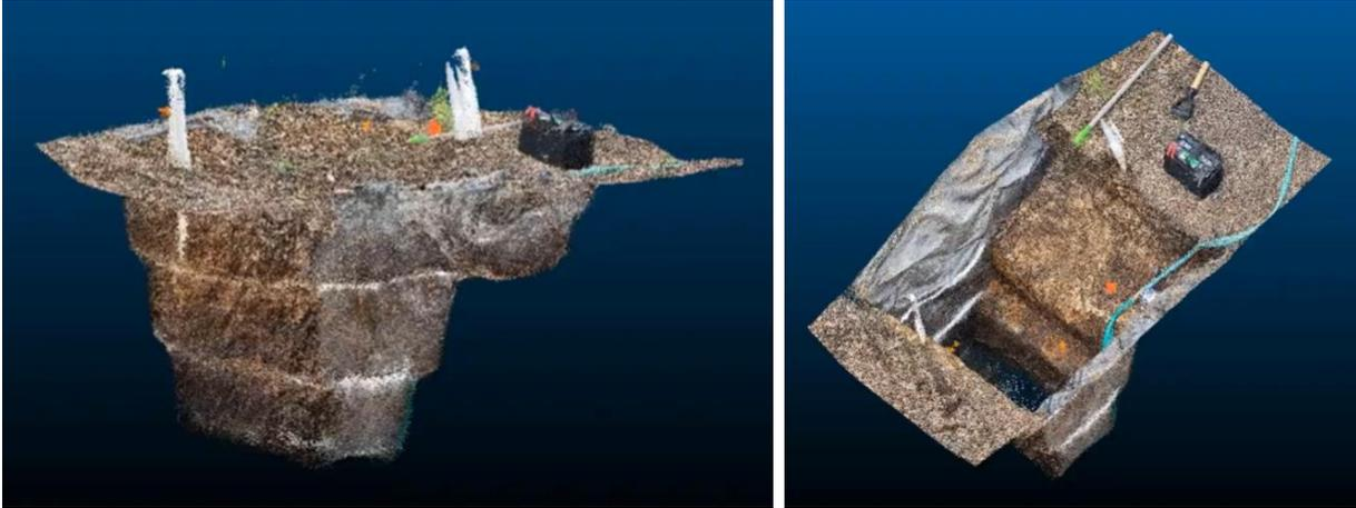
**Figure 2. iPhone LiDAR image of excavated UIUC Ag Engineering Farm pilot-scale woodchip bioreactor. The bioreactor was excavated to estimate how densely compacted the woodchips were after 2 years (that is, to determine the *in-situ* woodchip bulk density). See 41 second excavation video here: [https://mediaspace.illinois.edu/media/t/1\\_7qckhbm3](https://mediaspace.illinois.edu/media/t/1_7qckhbm3)**
