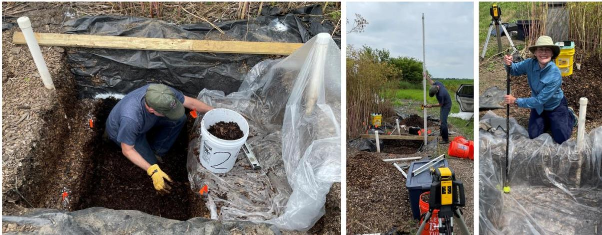
**Figure 1. Photo collage of summer 2021 excavation of a UIUC Ag Engineering Farm pilot-scale bioreactor to estimate *in situ* woodchip bulk density.**
