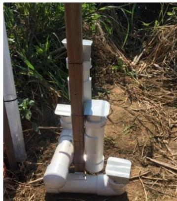
Image 1. New stacked pole samplers to be used in calculating trapping efficiency.
