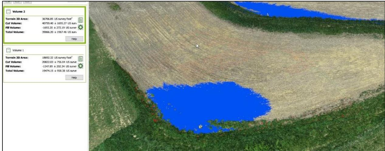
Image 5. Drone footage taken of WASCoB 1 (WASCoB CC) on May 24 will be used to calculate the total volume of each basin in the WASCoB. This is an image analyze by the Pix4Dmapper software.
