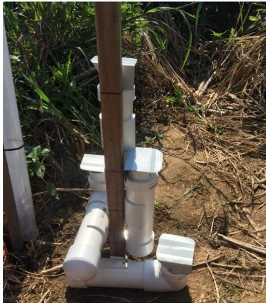
Image 1. New stacked pole samplers installed in each basin.
