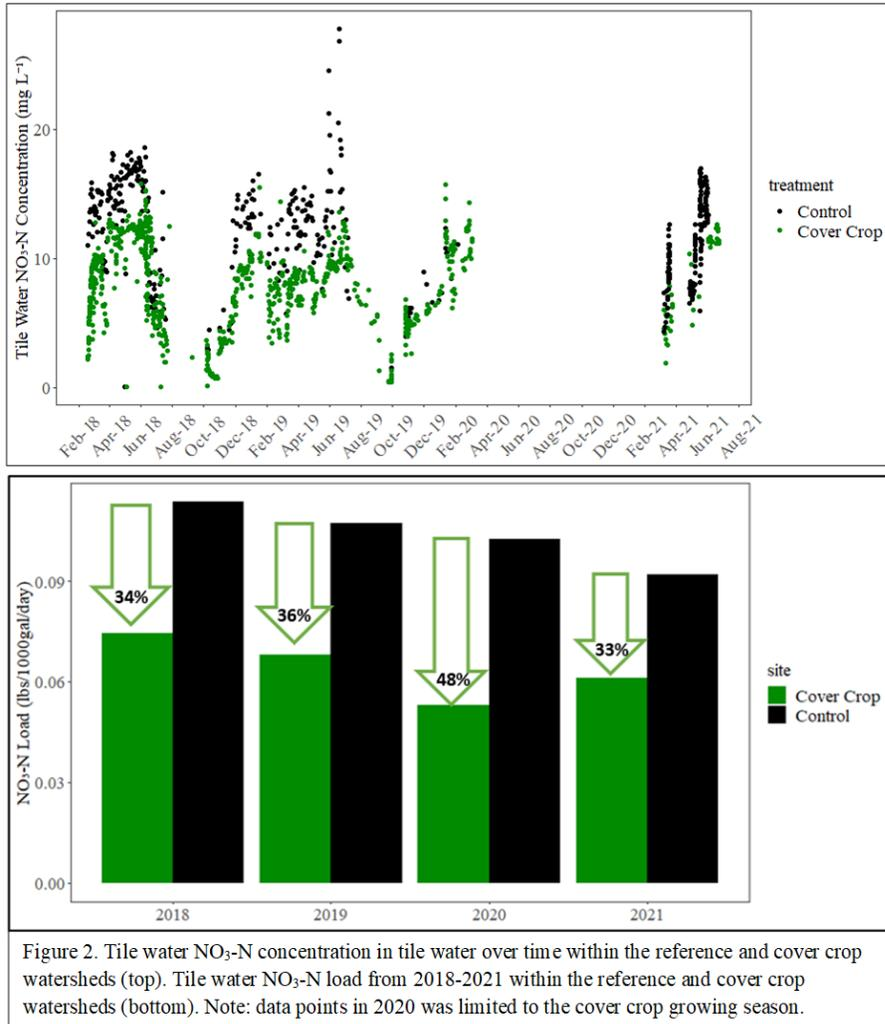
Figure 2. Tile water NO<sub>3</sub>-N concentration in tile water over time within the reference and cover crop watersheds (top). Tile water NO<sub>3</sub>-N load from 2018-2021 within the reference and cover crop watersheds (bottom). Note: data points in 2020 was limited to the cover crop growing season.
