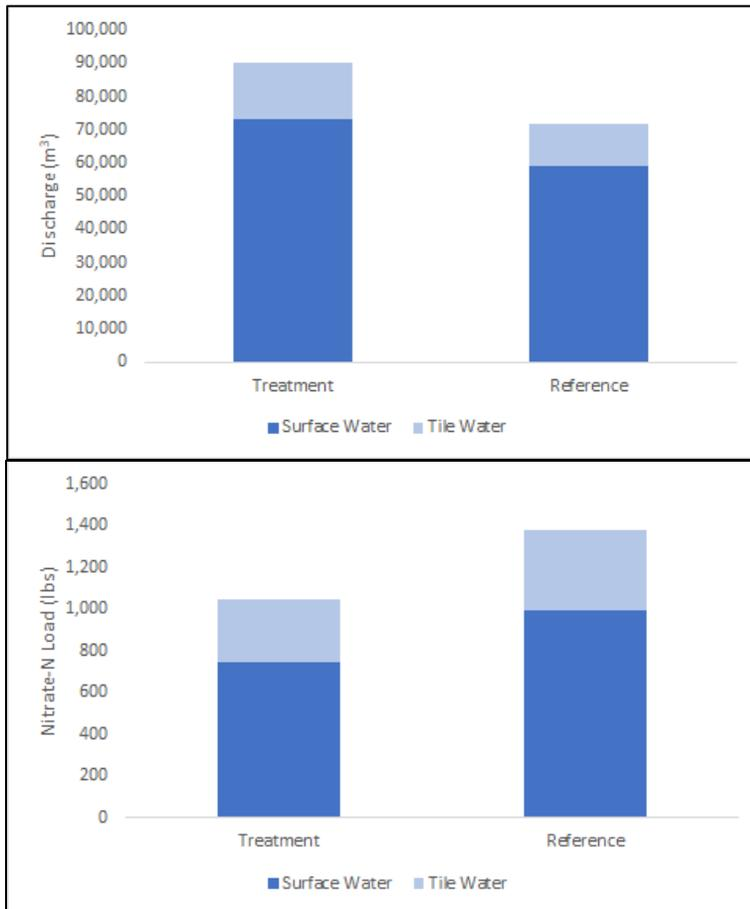
Figure 5. Discharge and nitrate-N load for surface and subsurface drainage within both reference and treatment watershed on July 9-12<sup>th</sup>.
