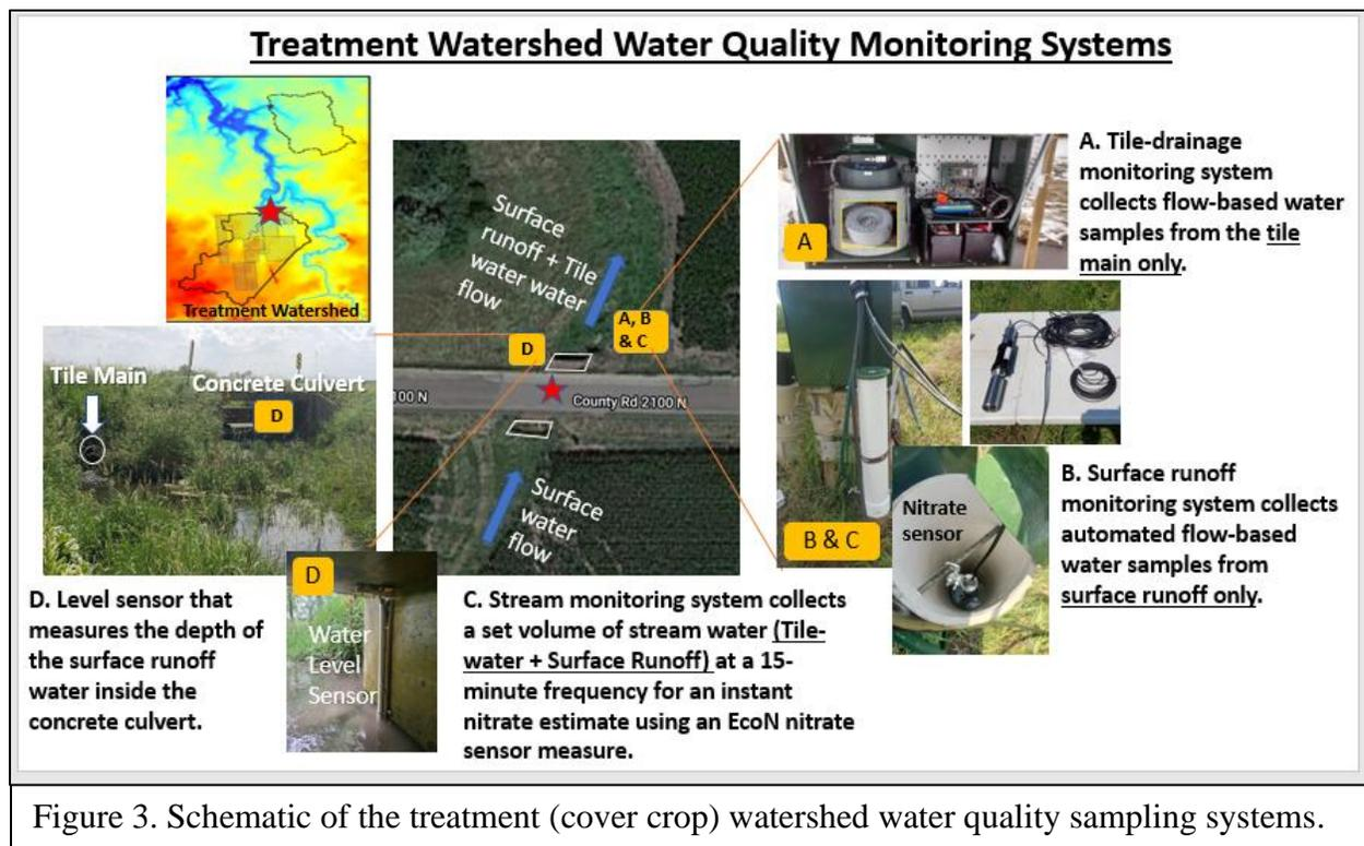
Figure 3. Schematic of the treatment (cover crop) watershed water quality sampling systems.
