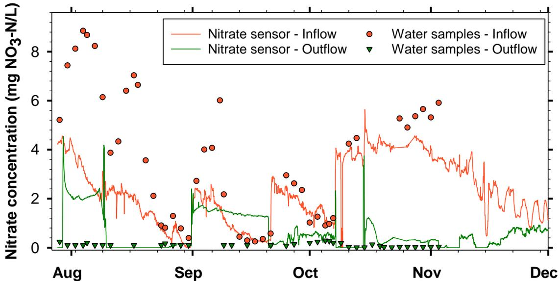
**Figure 2. Bioreactor inflow and outflow nitrate concentrations as collected by autosamplers and with high-frequency sensors at the UIUC ACES Dudley Smith Farm (Pana, Illinois). These data are preliminary and not for public distribution as there is a clear discrepancy between sampled and sensed nitrate concentrations. Further quality control and assessment will be performed in 2022.**
