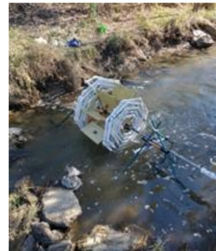
Field testing a double hexagonal pipe coil on the University Farm
