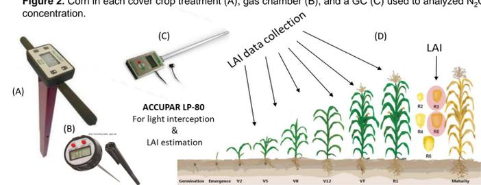
Figure 3. TDR 350 (A), soil thermometer (B), ACCUPAR LP-80 for measuring LAI (C) during the corn growth stages (D).
