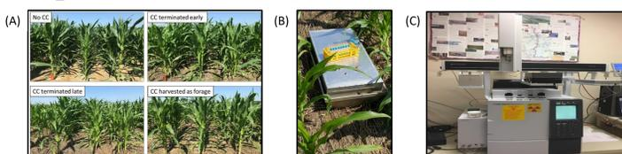
Figure 2. Corn in each cover crop treatment (A), gas chamber (B), and a GC (C) used to analyze N<sub>2</sub>O concentration.
