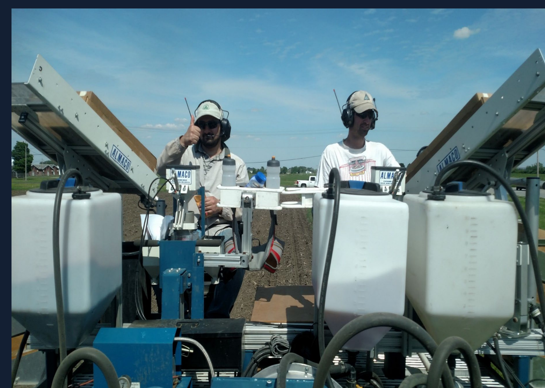
Figure 2. Planter-mounted Sure-Fire in-furrow system.
